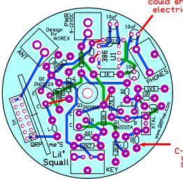
10uf cap pad closest to the edge of the board could short to the rim of the can. Use some electrical tape or similar item to insulate the pad
